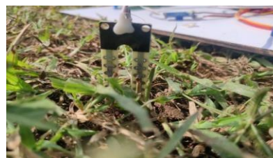
Fig:4.4.0 Inserting moisture sensor
