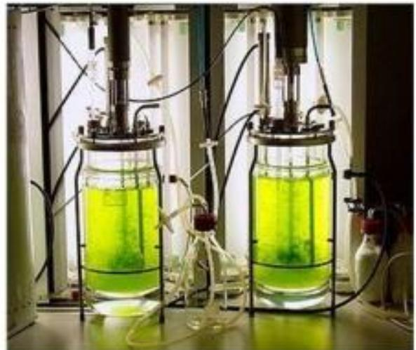
Further satisfactory entrance of daylight ought to be kept up with. The cylinders ought to likewise be cooled to forestall climb in temperature. Photograph bioreactors are generally worked in a constant mode at a temperature in the scope of 25-40°C. Microalgae and Cyanobacteria are regularly utilized. The creatures develop during sunlight while the items are delivered during night. Certain significant mixtures are delivered by utilizing photograph bioreactors e.g., p carotene, asthaxanthin.
