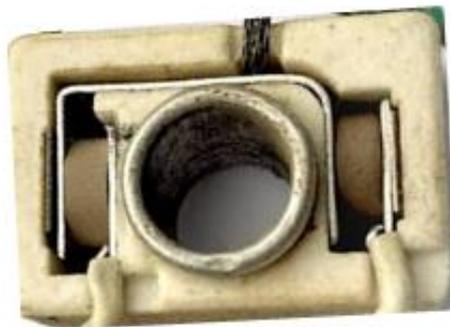
**Figure 15: Shows MQ 6 Sensor**
