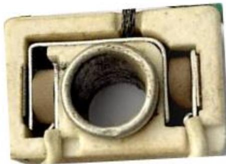
**Figure 15: Shows MQ 6 Sensor**
