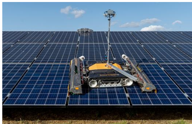
Figure7: Automatic Wiper Based Cleaning
