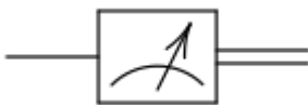
Circuit representation of measurement. The two lines on the right hand side represent a classical bit, and the single line on the left hand side represents a qubit.
