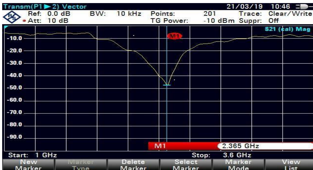
Figure 13 Measured result for isolation of integrated WPD
