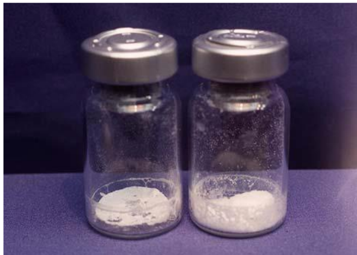
Figure 10. Collapsed Product – Critical Temperature was exceeded
