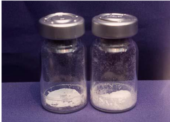
Figure 14. Collapsed Product – Critical Temperature was Exceeded
