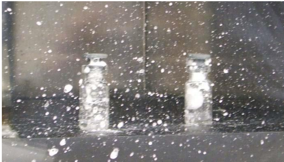
Figure 15. Product that was not fully frozen before starting vacuum & drying
