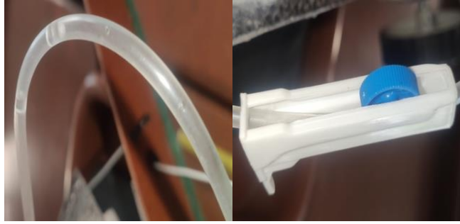
Figure 10: PVC Pipe and Flow Control Valve
