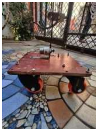
Fig. 4: Trolley to rotate the lift around Building
