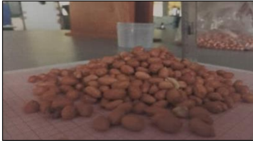
Fig .2. Angle of repose test of groundnuts.
