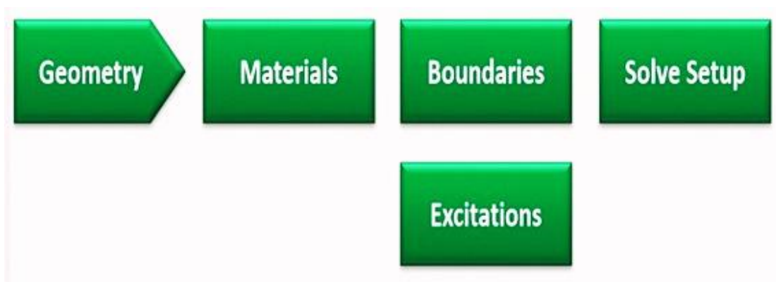
Figure 3.9: Design flow process of HFSS
