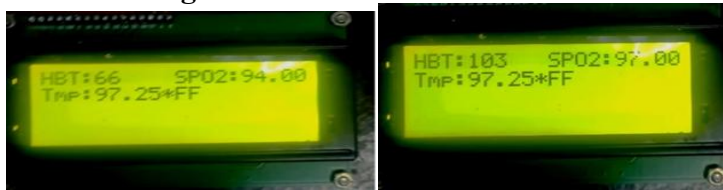
Fig. 4 Displaying body temperature, heart rate and Spo2 in LCD of different persons.
