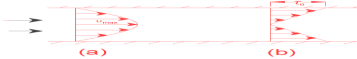
Figure 7.9 This diagram portrays the velocity and shear stress distribution along a section of parallel plates.
