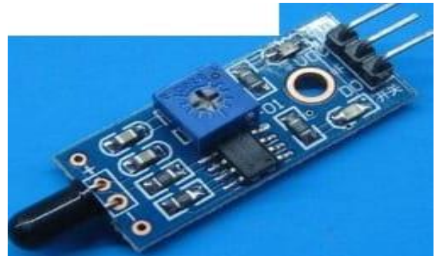
Figure 6: IR Fire sensor
