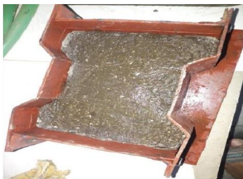
Fig:6 Added mixture into mould
