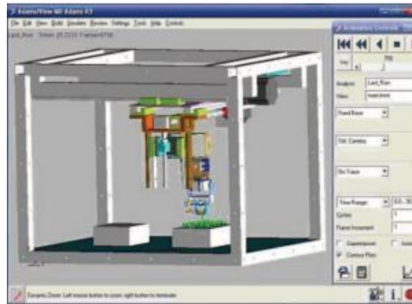
Fig 5: Robotic teeth arranger of the Cartesian kind, digital model.
