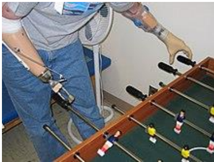
Fig. 1.6. Artificial limbs: The right arm is an example of a prosthesis, and the left arm is an example of myoelectric control.
