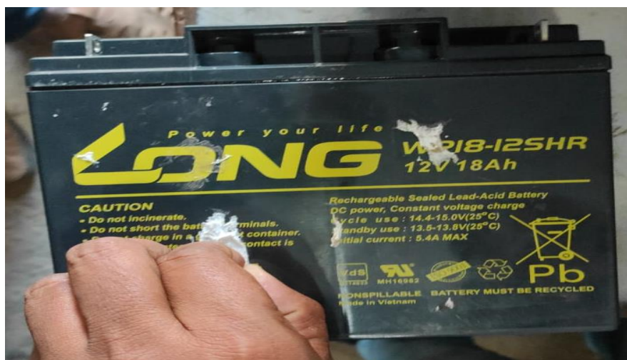
Fig.3 12v and 18 amps lead acid Battery
