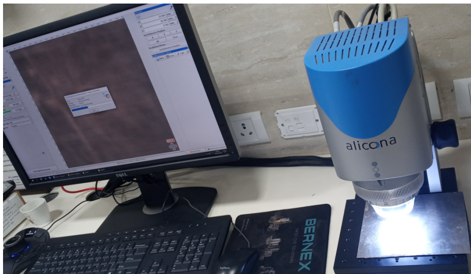
Fig.1 Measuring diameter of machined micro holes on work material by ALICONA optical microscope.
