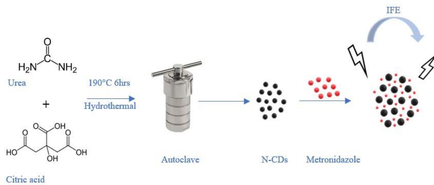
Fig 20. Schematic illustration of synthesis of N-CDs for the detection of metronidazole
