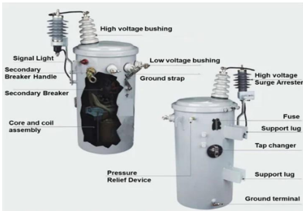
Figure 1. The basic structure of distribution transformer
