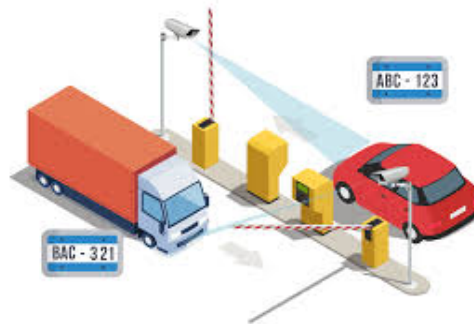
Fig 2: Automatic Number Plate Recognition (ANPR) with barrier gate [www.vdttechnology.com]
