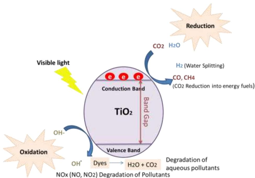
**Figure 4:** Photocatalytic applications of TiO<sub>2</sub> nanostructures
