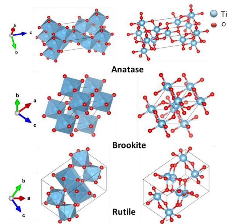
**Figure 1:** Different crystal forms of TiO<sub>2</sub>
