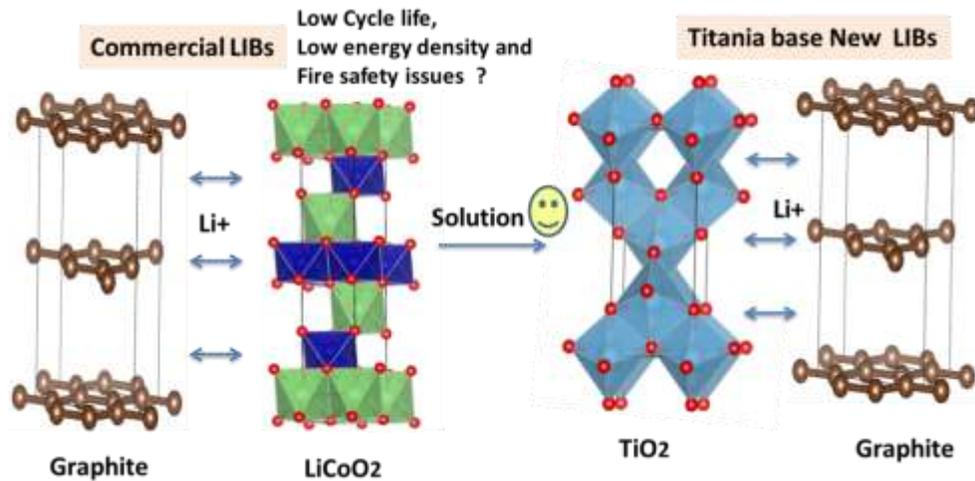
**Figure 6:** Titania based nanostructures as electrodes in lithium ion batteries
