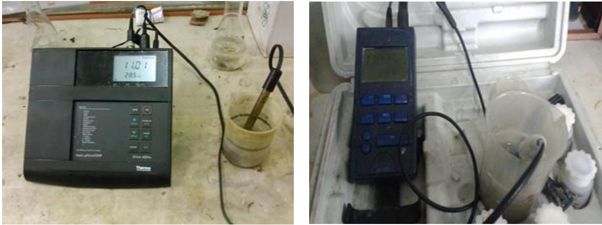
Figure 11. pH value determination of RHA blended OPC and PPC
