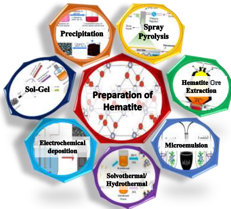
Figure 8. Various hematite preparation processes. [51,76–80].
