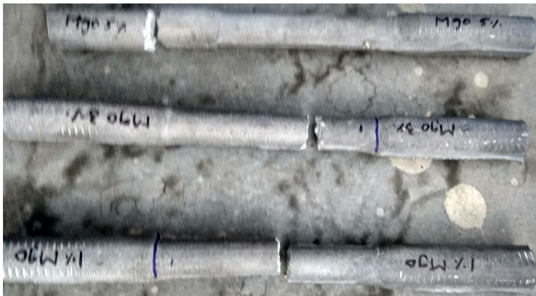
Figure 4.6: Actual samples of LM 25 + 1%, 3% and 5% MgO after tensile test
